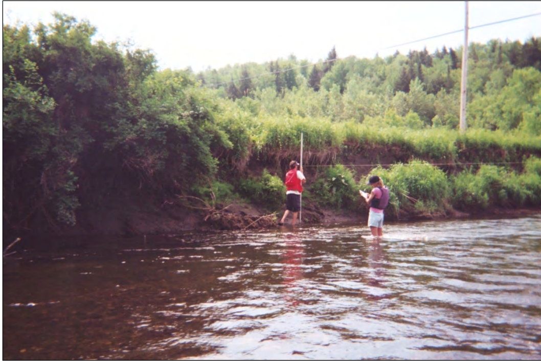
Figure 14. R23-A has undergone historic channel degradation. The incision ratio, illustrated in this photograph, was recorded at 1.5. Major disturbance of the riparian buffer is also evident in this photograph.
